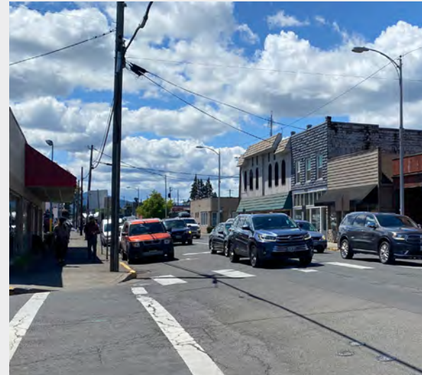
Many crossings of 12th St and 13th St can be hazardous for children and adults alike. At this crossing of 12th St at Pine St, parked cars block northbound drivers from seeing pedestrians enter the crosswalk until they are already driving through.
